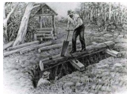
Woodcut showing work above a saw pit
