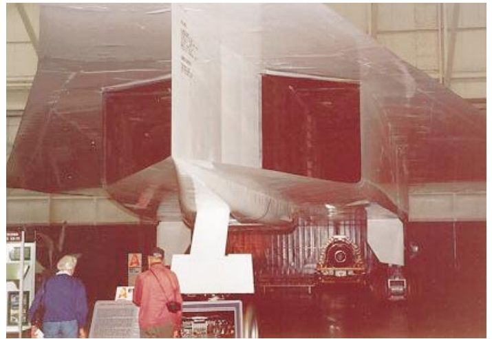
The Massive intake ports of the XB-70 engines
