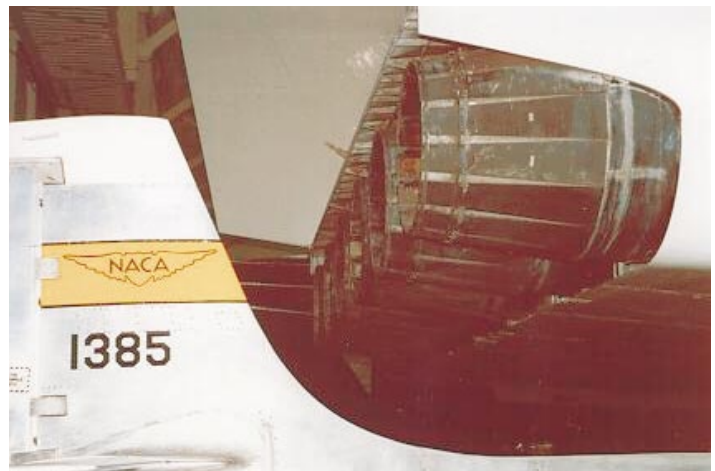
The six exhaust nozzles of the XB-70's huge jet engines
